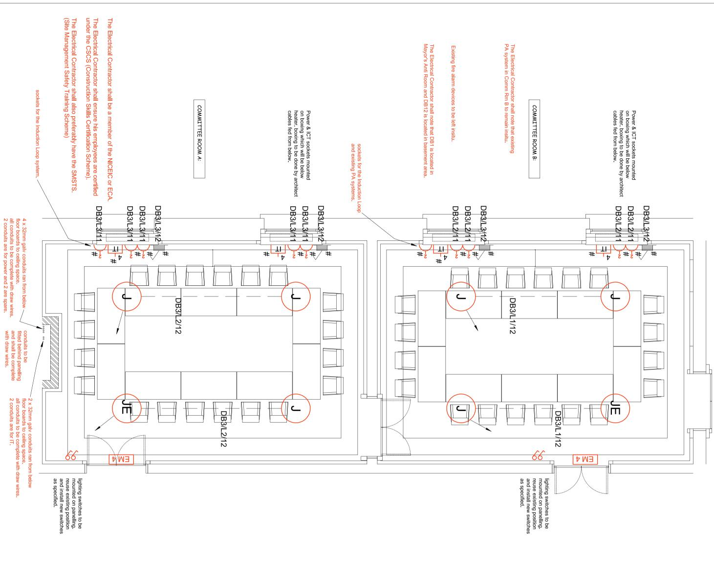
ltg r/m ccts radial cct for fan convectors electrical contractor to supply and install suitably rated m.c.b.'s into this d.b. for these circuits. - 6amp R.C.B.O. lighting and power circuits to be taken from d.b.3 located in Members Suite Kitchen. - 32amp 30mA - 10amp
